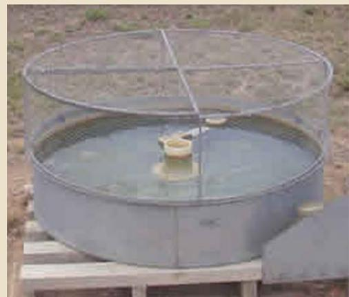
Evaporation is measured, in millimetres of water, using an evaporation pan. It is an open pan of water and is covered with bird netting to stop birds and animals drinking from it. Evaporation is determined by measuring the amount of water required to refill the pan to a predetermined level.
