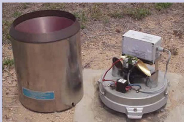
At automatic weather stations a 'tipping bucket' rain gauge is used to measure rainfall. The rain that lands in the funnel drips into one side of a double 'bucket' on a balance. Each bucket holds a specified amount of water. When one bucket fills, it overbalances, recording one 'unit' of rain, emptying itself, and the second bucket begins to fill.
