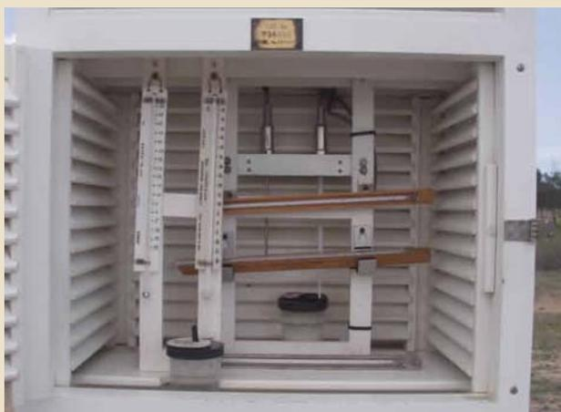
Thermometers to measure temperature, including minimum, maximum, and wet bulb and dry bulb for relative humidity are located in a 'Stevenson Screen' situated 1.2 m above ground level. The screen protects the thermometers from direct sunlight but allows good air flow. A frost is defined as when the screen temperature drops below 2 °C.
