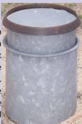
Ideally a rain gauge should be placed so that the lip of the gauge is 30 cm above ground level, in a clearing away from obstructions such as trees and buildings. The Australian Bureau of Meteorology specifies: a rain gauge should not be placed closer to an obstruction than four times the height of that obstruction. For example, if there is a 10 m high tree nearby, the rain gauge should be placed at least 40 m from it.
