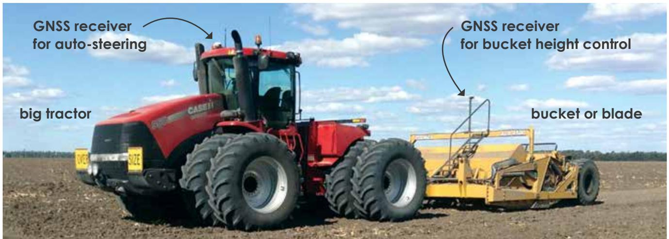
The components of a GNSS levelling system.
