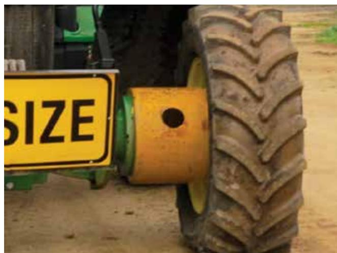
Cotton-reel spacers are used to spread the front axle of tractors to 3m centres. The image on the left is a John Deere spacer which is warranted. The one on the right shows a locally engineered retrofitted version.
